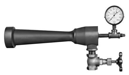
The Eclipse AirJector uses compressed air to entrain larger volumes of ambient air for combustion systems. For systems using the gas stream to entrain air, reference Atmospheric Injectors in catalog section 650.
