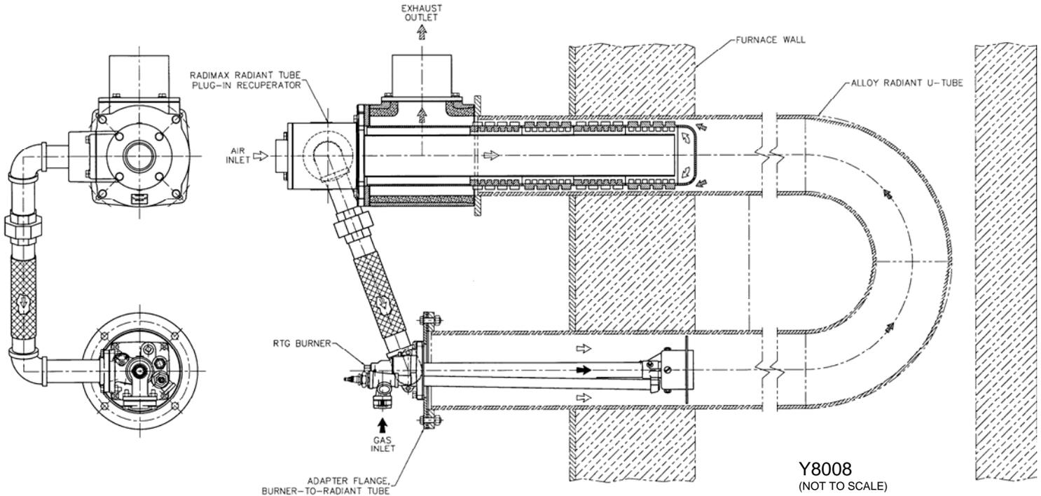
**Figure 9. Typical Installation of RADimax Radiant Tube Plug-In Recuperator**
