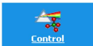
Clicking on this symbol leads to the following display which branches to functions “Calibration”, “Verification” and “Disable touch”.
