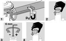
**5** Clearly mark the adjusted value of the outlet pressure p<sub>d</sub> on the type label.
