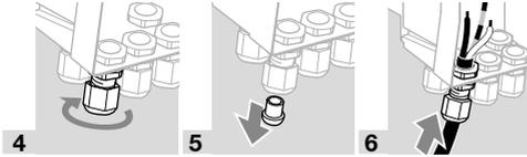
**7** Secure used cable glands. Tightening torque: max. 3.5 Nm.
