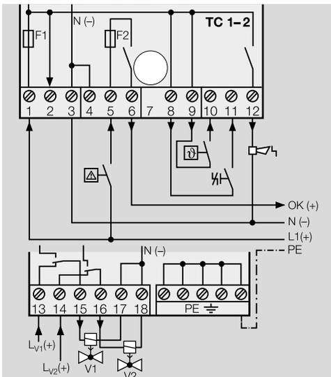
Mains voltage: 120 V AC/230 V AC, control voltage:
