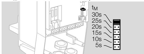
→ No jumper: no function. The operating signal LED  $\overline{V}$  is permanently red, see page 8 (9 Assistance in the event of malfunction).
