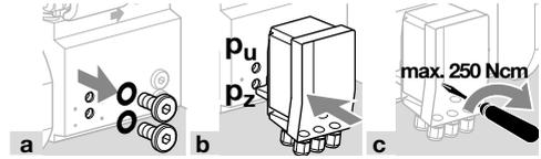
→ Tighten the screws with max. 250 Ncm.
