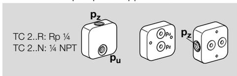
→ We recommend using Ermeto screw couplings to attach the adapter plate to the gas solenoid valve. It may be necessary to compensate the distance to the valve housing.
