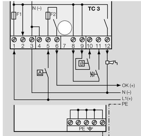
Mains voltage: 120 V AC/230 V AC, control voltage: 24 V DC
