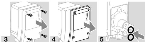
→ The O-rings must be inserted in the connectors of the TC.
