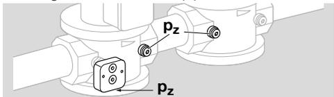
→ Ensure that connections  $p_u$  and  $p_z$  on the TC and adapter plate are not reversed.
