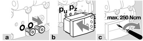
→ Tighten the screws with max. 250 Ncm.
