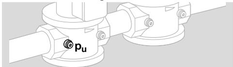
→ Only use approved sealing material to seal the pipe connections.
