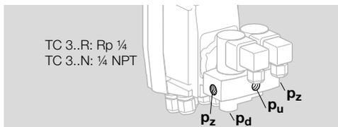
→ Use a 12 x 1.5 or 8 x 1 pipe for the pipe connections.
