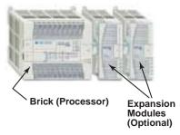
Allen Bradley Micrologix 1200 (expandable PLC) Integrated Logic Control
