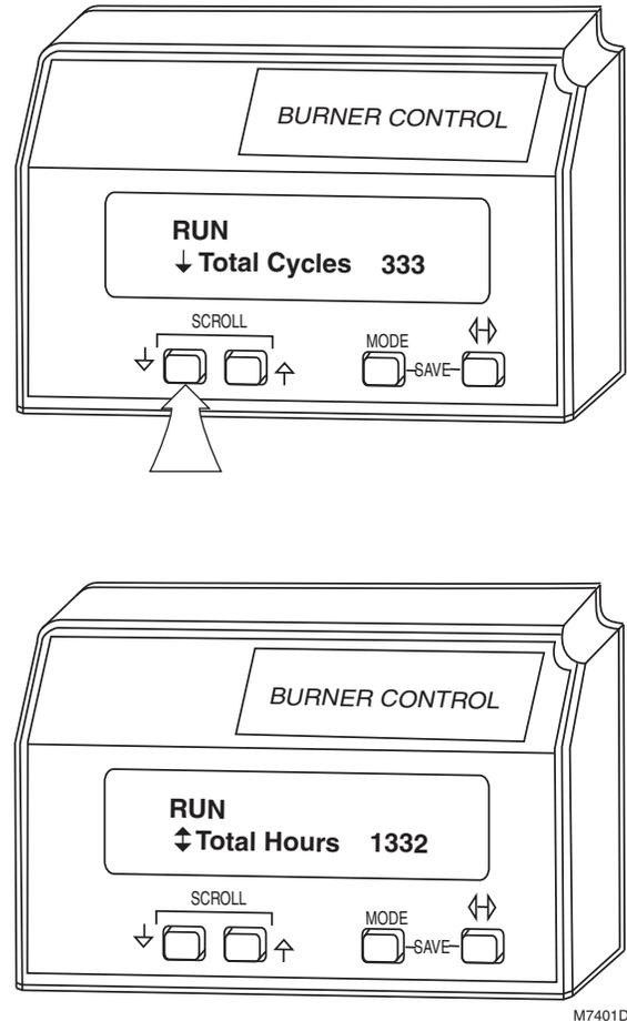
Fig. 19. SCROLL pushbutton function.
