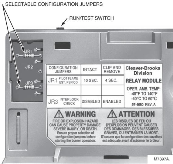
**Fig. 23. Selectable site-configurable jumpers.**
