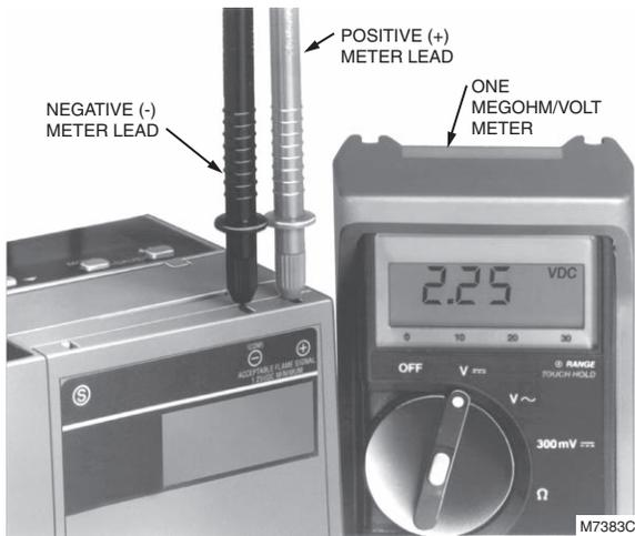
**Fig. 24. Flame signal measurement.**
