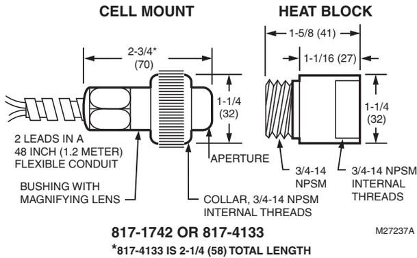
**Fig. 5. Infrared detector, mounting dimensions in inches (mm).**
