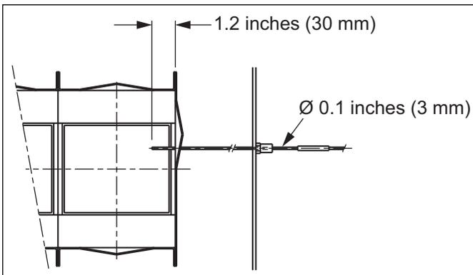
**Figure 5.2. Thermoelement Detail
