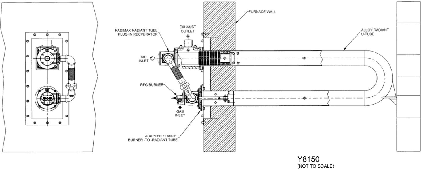
**Figure 2. Typical Installation Radimax Plug-In Recuperator W/RADiflame Gas Burner**
