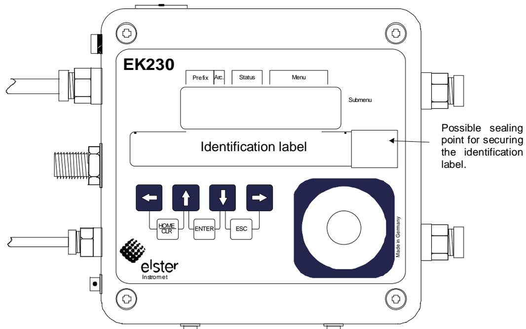
**c) Housing cover (front view), cover sealing using wire seal (optional user sealing)**
