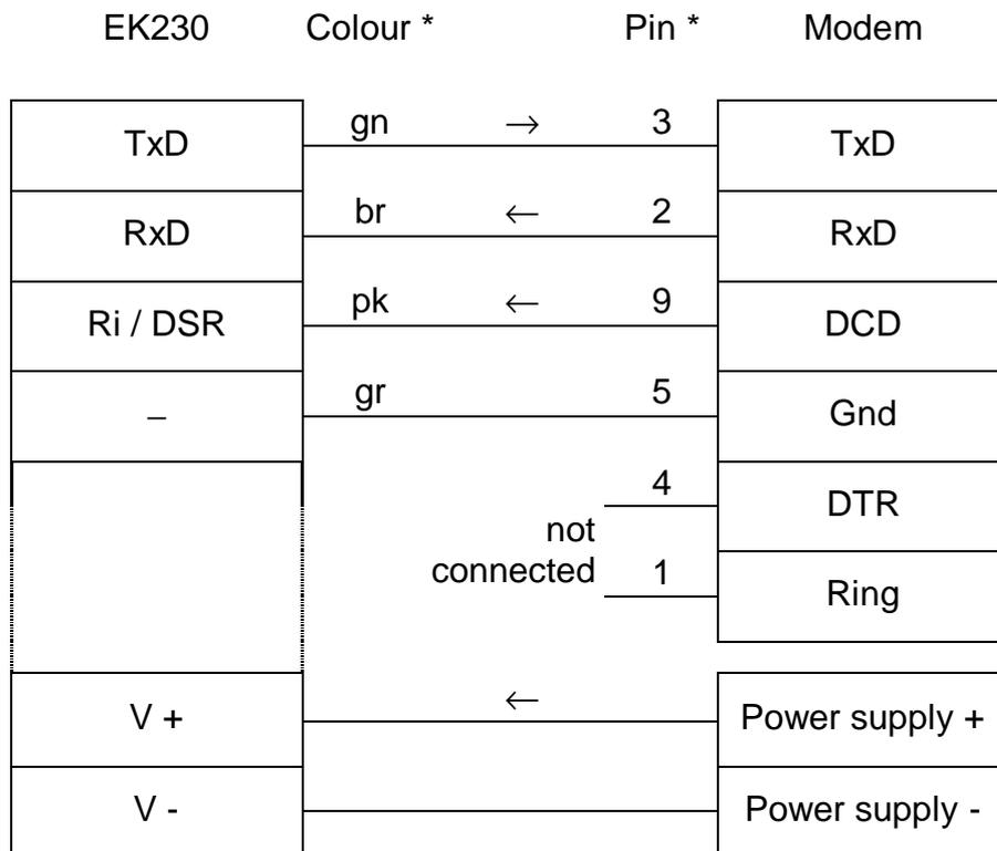
\* Pin numbers of the DSUB-9 plug and core colours when using a ready-made cable available from Elster GmbH, e.g. Order No. 73016923 (2 m) or 73017268 (10 m).
