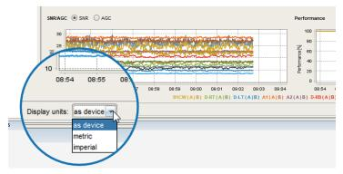
Fig. 4-2: Determine the units used in the dashboard
