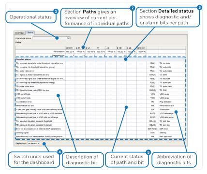
Fig. 4-4: Tab Status breaks down diagnostic data per path
