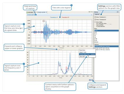
Fig. 10-2: Signal capture graph view with filter settings - example
