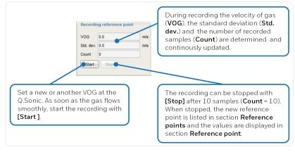
9-3: Controls and fields in section Recording reference point
