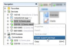
Fig. 8-1: Calling the action "Creating a support package" via the context menu – example with 2 meters selected
