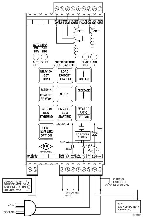
Fig. 1. Model 700ACSP Signal Processor Wiring.
