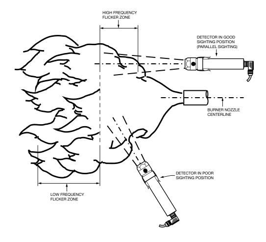
Fig. 16. IR Viewing Head Location
