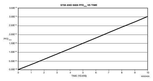
Fig. 30. Dependence of the PFD $_{\Delta VG}$  on the proof test interval for S706 & S806.
