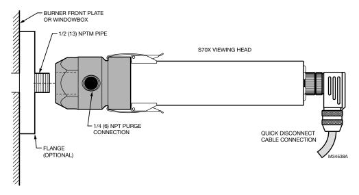
Fig. 15. Viewing Head Mounting Example.
