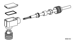
Fig. 7. ASY786 Viewing Head Plug Assembly with C330S.
