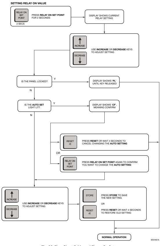
Fig. 23. Flow Chart 5: Manual Flame On Setup.
