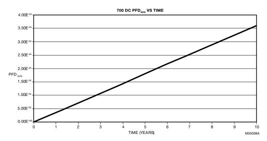
Fig. 29. Dependence of the PFD<sub>AVG</sub> on the proof test interval for 700DC.
