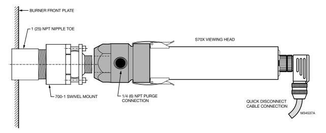
Fig. 14. Viewing Head Mounting Example.
