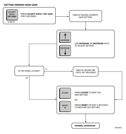
Fig. 27. Flow Chart 9: Viewing Head Gain Setting.
