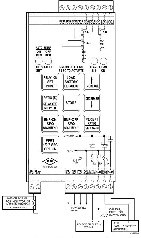
Fig. 2. Model 700DCSP Signal Processor Wiring.
