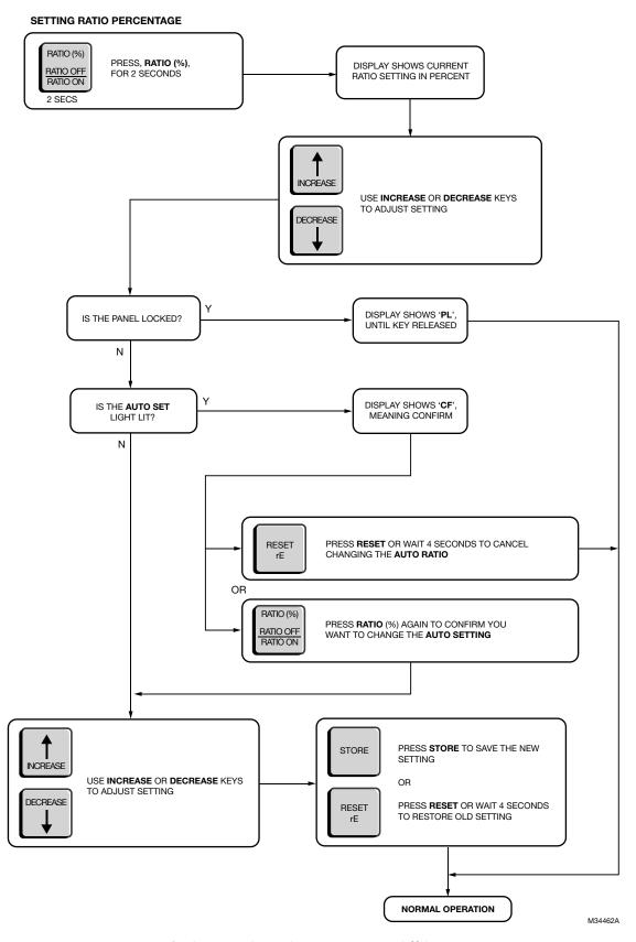
Fig. 24. Flow Chart 6: Manual Flame Off Setup.
