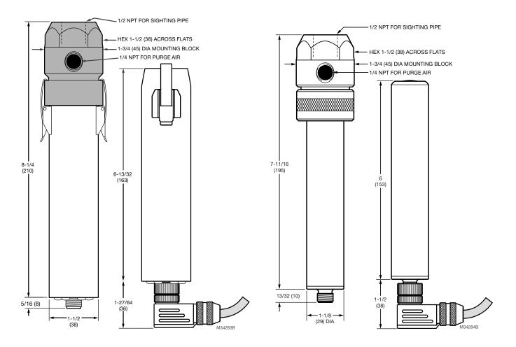
Fig. 10. Models S702 and S706 Viewing Heads.
