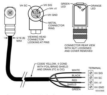
Fig. 4. Model 700/800 Viewing Head Cable Connections.
