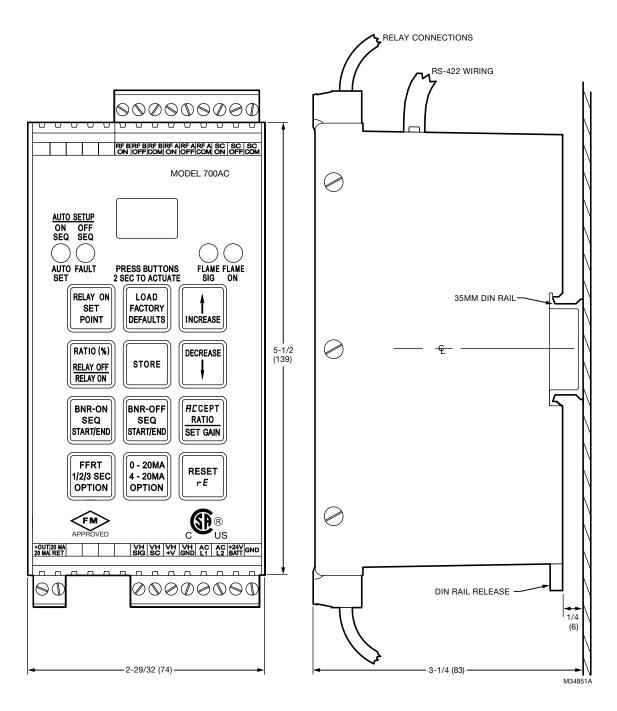
Fig. 13. Model 700ACSP Signal Processor.
