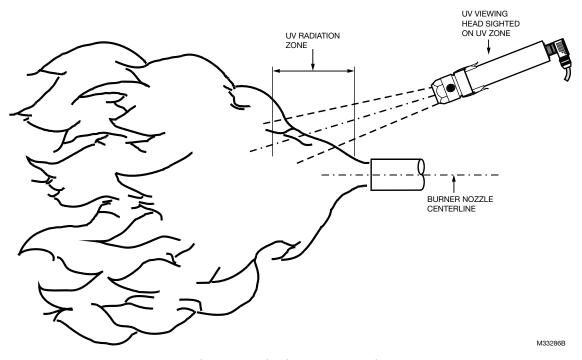
Fig. 17. UV Viewing Head Location
