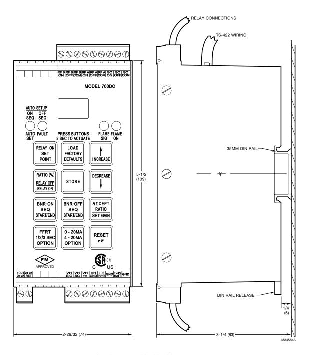
Fig. 12. Model 700DCSP Signal Processor.
