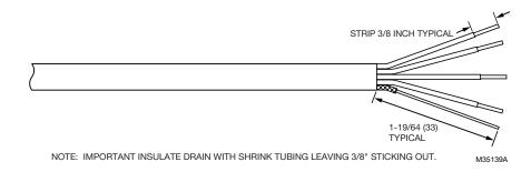
Fig. 5. C330S Signal Processor End Cable Preparation.
