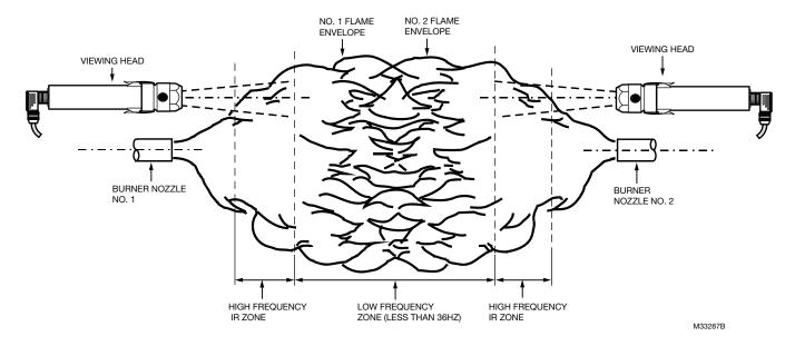
Fig. 18. Opposed Fired Viewing Head Sighting
