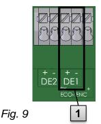
The pulse transducer of the gas meter is connected to the DE1 (1) terminal of the EK205.
