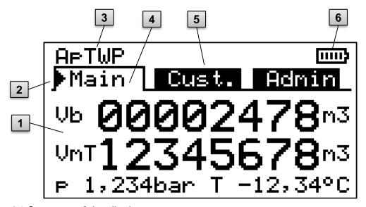
Fig. 21 Structure of the display
