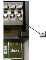
Connect the power supply to the "Uext" terminal 1 of the EK205.
