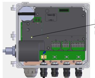
Position of the key for opening the calibration lock.
