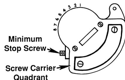
This minimum stop screw creates a mechanical block which prohibits the screw carrier quadrant and its direct-connected air butterfly valve from closing completely. Thus a "minimum" volume of fuel is allowed in through the control valve to the burner(s). This becomes the minimum gas pressure.
