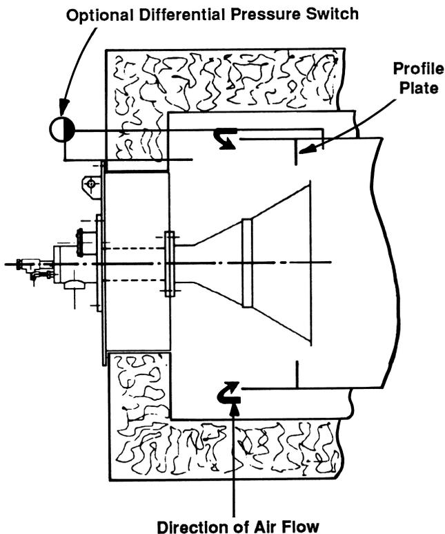
The Circular INCINO-PAK® Burner is used only for the heating of air in motion. It should be mounted so as to direct its flame **parallel to and in the same direction** as the **movement of the air** which is to be heated.
