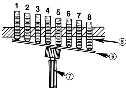
Removing a cover strip reveals a numbered series of adjusting screws ⑤ which bear on a set of cam strips ⑥ beneath the quadrant (see sketch above).
