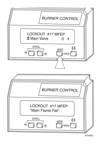
Fig. 21. MODE pushbutton function.
