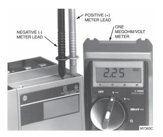
Fig. 24. Flame signal measurement.
