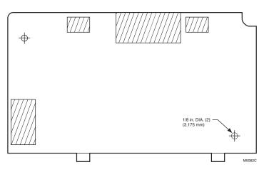
Fig. 26. Flush mounting of a Keyboard Display Module template.
