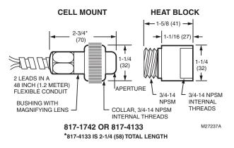
Fig. 5. Infrared detector, mounting dimensions in inches (mm).
