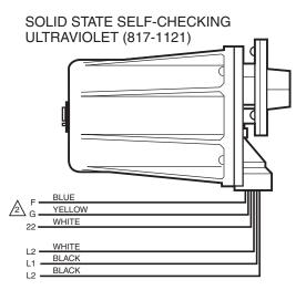
FLAME DETECTOR LEADS ARE COLOR CODED. THE BLUE LEAD MUST BE CONNECTED TO THE F TERMINAL AND THE WHITE MUST BE CONNECTED TO THE G TERMINAL. THE UV SENSING TUBE IS POLARITY SENSITIVE. REVERSING THE LEADS EVEN MOMENTARILY CAN DAMAGE OR DESTROY THE UV TUBE.
