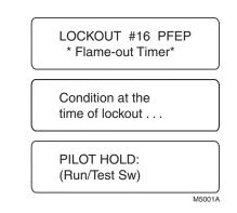
Fig. 25. Flame-out timer lockout.
