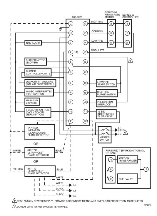
Fig. 7. Wiring the CB780/CB784 Relay Module.
