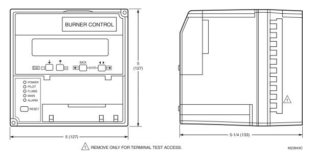
Fig. 1. Mounting dimensions of CB780/CB784 Relay Module and 833-2725 Subbase, in inches (mm).
