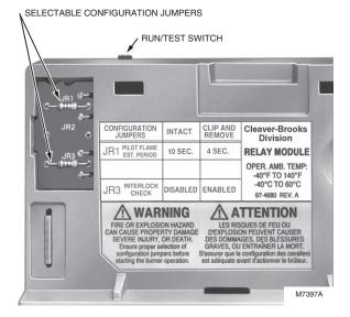
Fig. 23. Selectable site-configurable jumpers.
