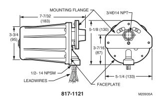
Fig. 3. Ultraviolet Self-Check detector, mounting dimensions in inches (mm).
