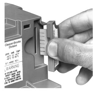
Fig. 11. Purge card installation.
