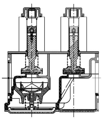
Fig. 8. Servo pressure regulator working
