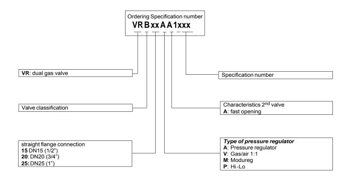
NOTE: Flanges to be ordered separately (see **Flange kits**) Pressure switch (Min. C60VRB00 serie) is standard included (C6097 on request available)(position has to be specified, see table NO TAG on NO TAG.
