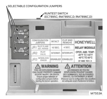
Fig. 6. Selectable site-configurable jumpers.
