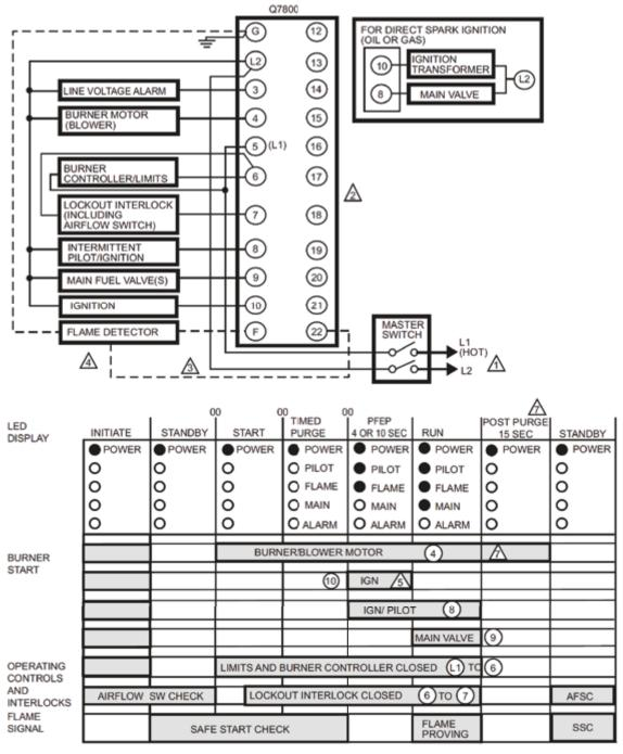
ARM7895, RM7896: 120 VAC, 50/60 HZ; EC7895: 220-240 VAC, 50/60 HZ POWER SUPPLY. PROVIDE DISCONNECT MEANS AND OVERLOAD PROTECTION AS REQUIRED.
