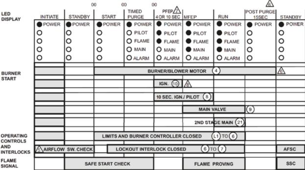
AN RM7895, RM7896: 120 VAC, 50/60 HZ; EC7895: 220-240 VAC, 50/60 HZ POWER SUPPLY. PROVIDE DISCONNECT MEANS AND OVERLOAD PROTECTION AS REQUIRED.
