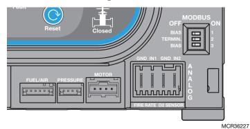
Fig. 2. Fuel Air Ratio Module connector location.
