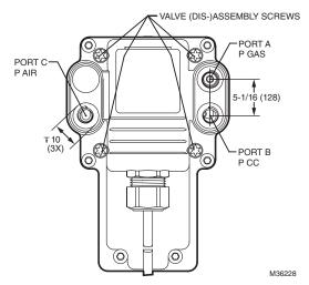
Fig. 3. Fuel Air Ratio Module pulse line connections
