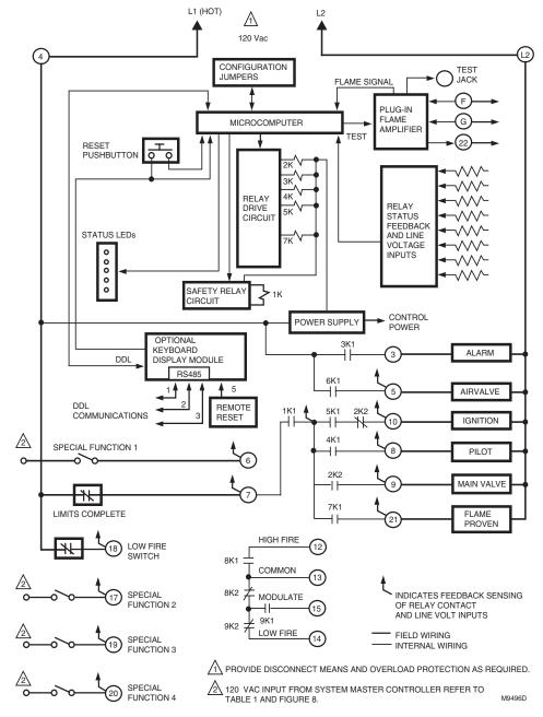
Fig. 10. RM7888A internal block diagram.
