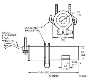
Fig. 7. Ultraviolet detectors (minipeepers).
