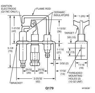
Fig. 2. Rectification detectors.
