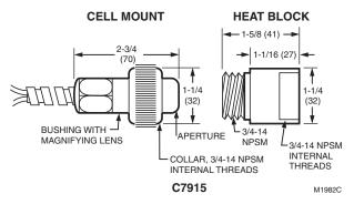
Fig. 4. Infrared detector.
