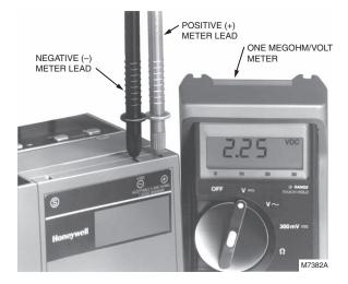
Fig. 25. Flame signal measurement.
