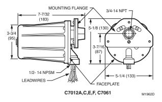
Fig. 3. Rectification detectors.
