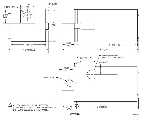
Fig. 8. Ultraviolet detectors (minipeepers).
