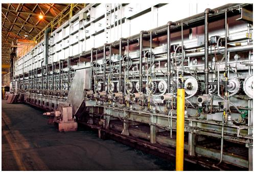
Roller Hearth Furnace - Drive Side. (Guards removed for photo to enhance visibility.)
