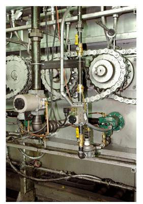
TJ Burner set up for high/low pulse firing
