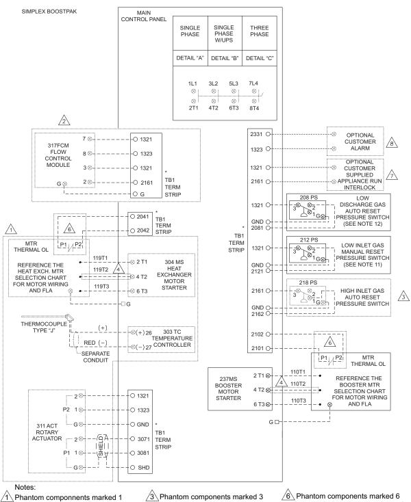
Phantom Components Marked 2 are installed on BoostPak models with the flow control option. The flow control contact is set to close when gas fired equipment causes flow.
