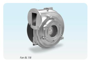
In condensing boilers, the speed-controlled fan BL distributes the mixture of gas and air required for the combustion process evenly over the surface of the radiant burner so that it can be combusted perfectly.
