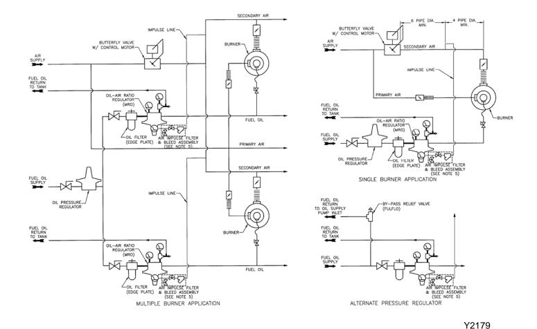
NOTE: 1. RELIEF VALVE ON OIL-AIR RATIO REGULATOR IS PRE-SET AT 75 PSIG (517 KPA).
