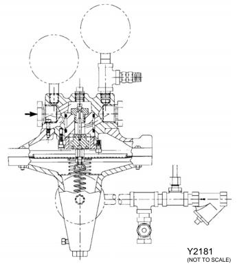
Figure 1. MRO Regulator With Optional Air Impulse Filter and Bleed Assembly
