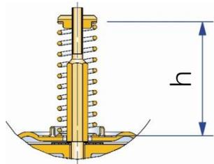
7. Remove diaphragm assembly (Full Relief) (23) or (Limited Relief) (35), and relief assembly from the diaphragm case (17).
