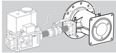
Integrated gas/air 1:1 with venturi mixing unit, see instruction sheet VMU "Mixing unit for V473xC/ V8743xC gas controls" (65-0282) [www.docuthek.com](http://www.docuthek.com).
