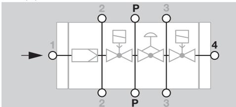
5 Install the leak test tap into pressure tap point **P** on the valve body.
