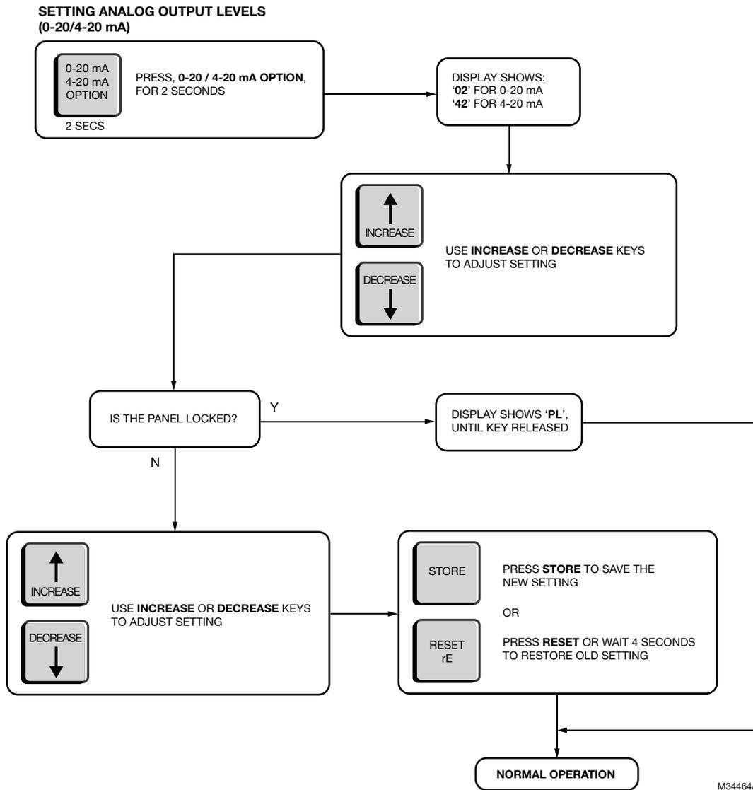
Fig. 26. Flow Chart 8: 0-20/4-20mA Analog Output Setup.
