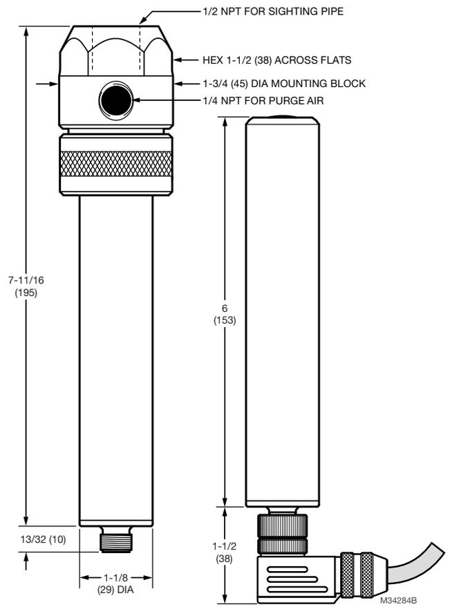
**Fig. 11. Models S802 and S806 Viewing Heads.**
