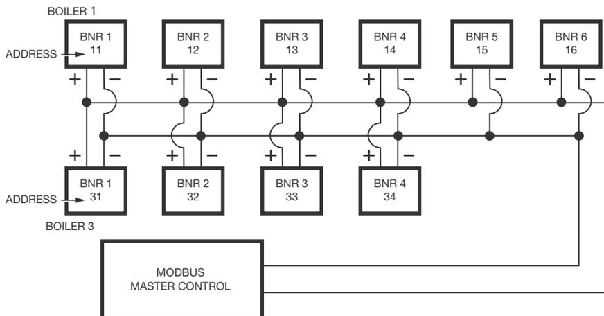
NOTES: A CONVERTER MAY BE NECESSARY FOR COMMUNICATION WITH THE MODBUS MASTER CONTROL.
