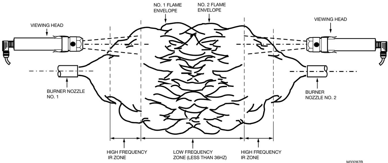
**Fig. 18. Opposed Fired Viewing Head Sighting**
