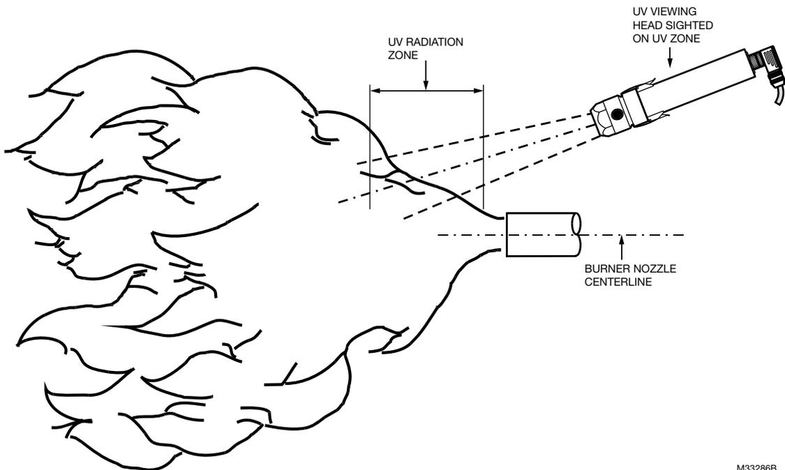
**Fig. 17. UV Viewing Head Location**
