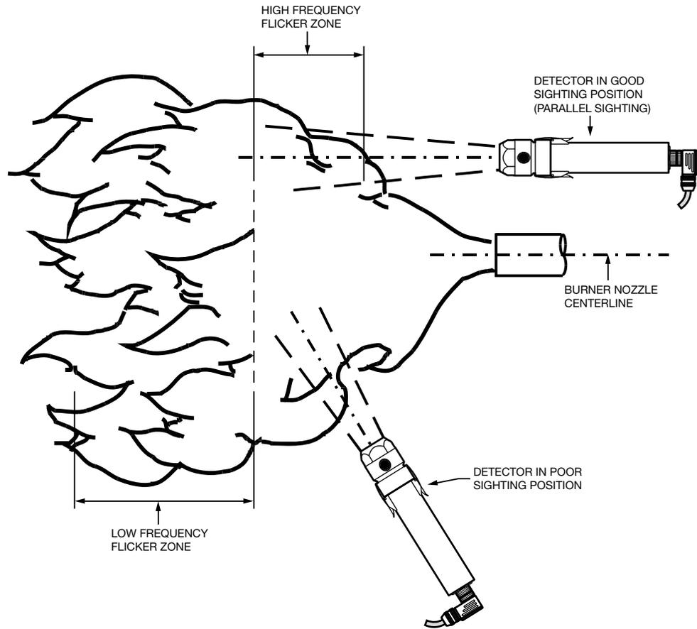
**Fig. 16. IR Viewing Head Location**
