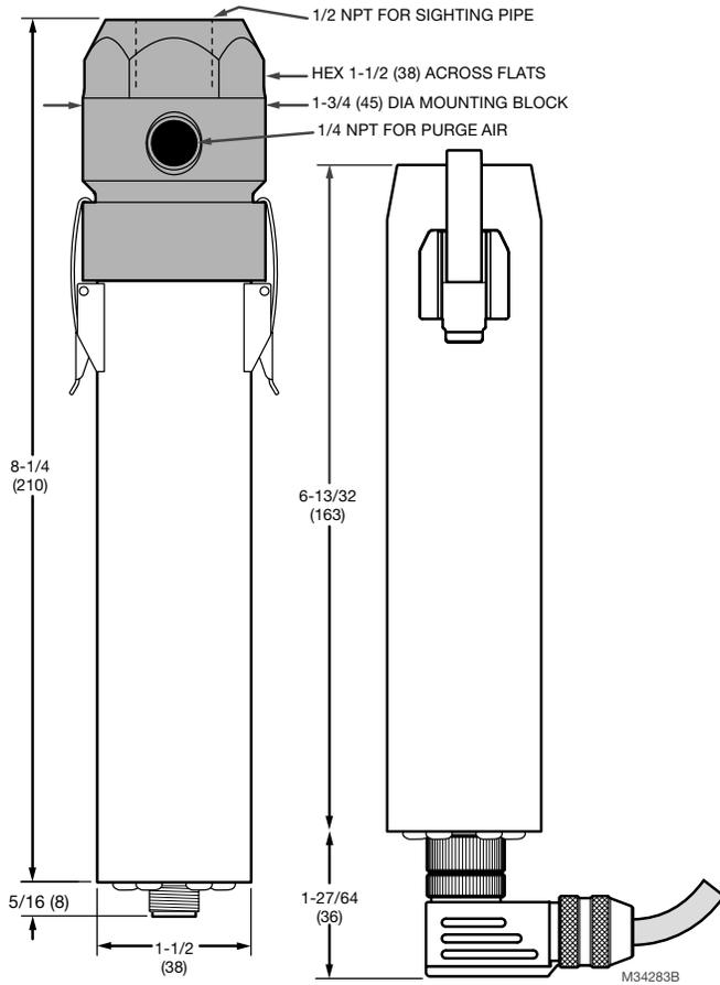
**Fig. 10. Models S702 and S706 Viewing Heads.**
