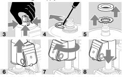
→ In both connection boxes, push through the knock-out for the cable gland set – then remove the covers. The covers must not be taken off before pushing through the knock-outs as it prevents damage to the connection boxes.
