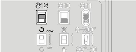
cw (blue mark on the cover) = valve opens clockwise,
