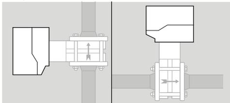
→ Do not insulate the actuator with thermal insulation.
