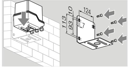
The actuator can be attached to a solid structure using the wall mounting bracket.
