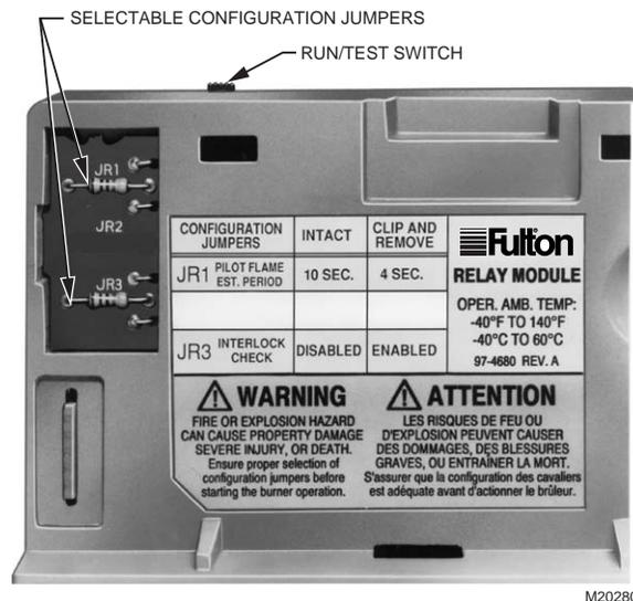
Fig. 27. Selectable site-configurable jumpers.
