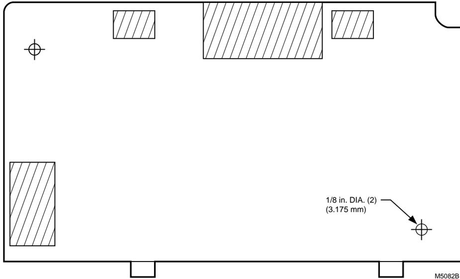
Fig. 30. Template for flush-mounting a Keyboard Display Module.
