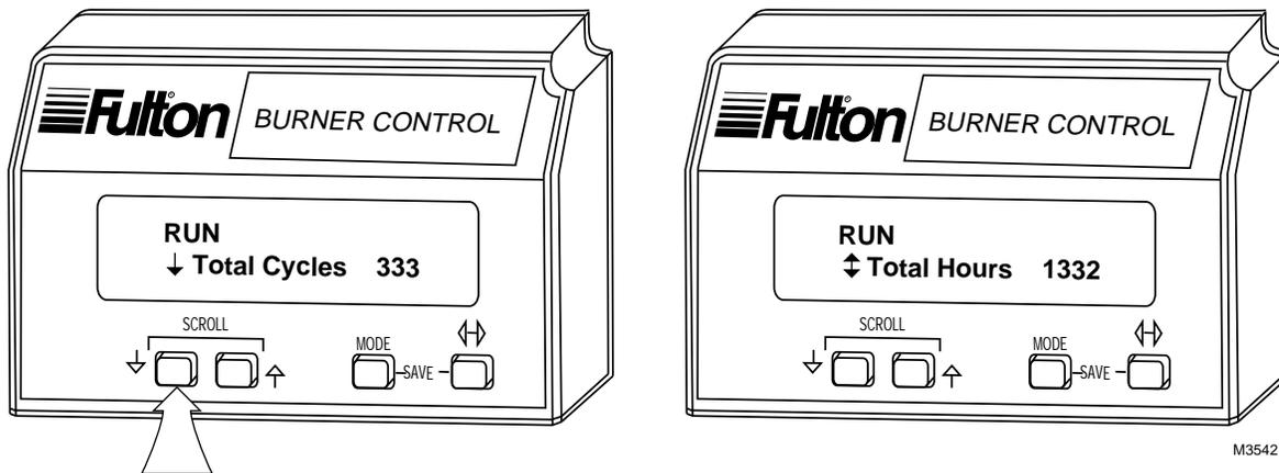
Fig. 23. (P) SCROLL pushbutton function.
