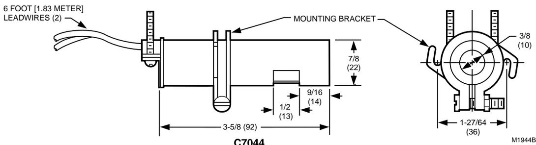
Fig. 4. Ultraviolet detectors.
