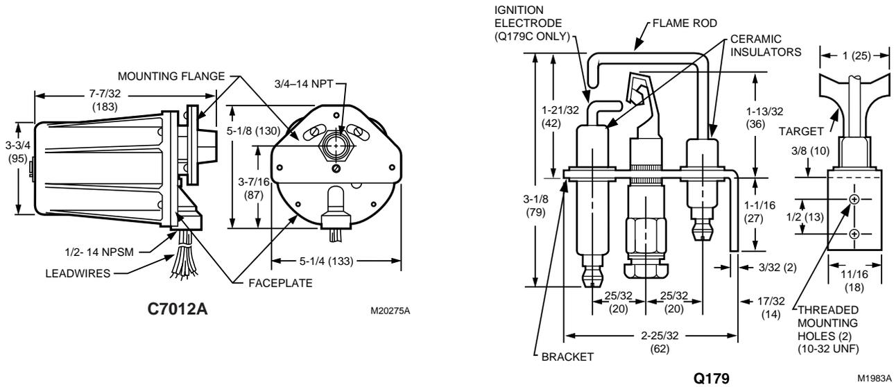
Fig. 3. Rectification detectors.
