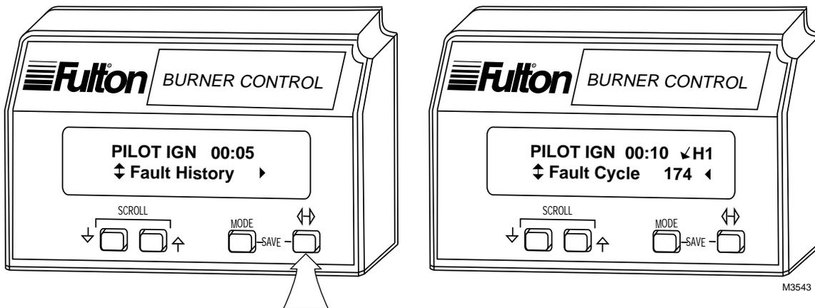
Fig. 24. (↔) Change-Level pushbutton function.
