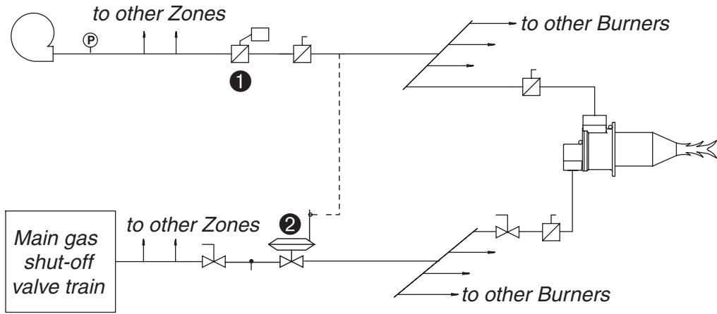
*Figure 1: Typical amplitude-modulated combustion system*
