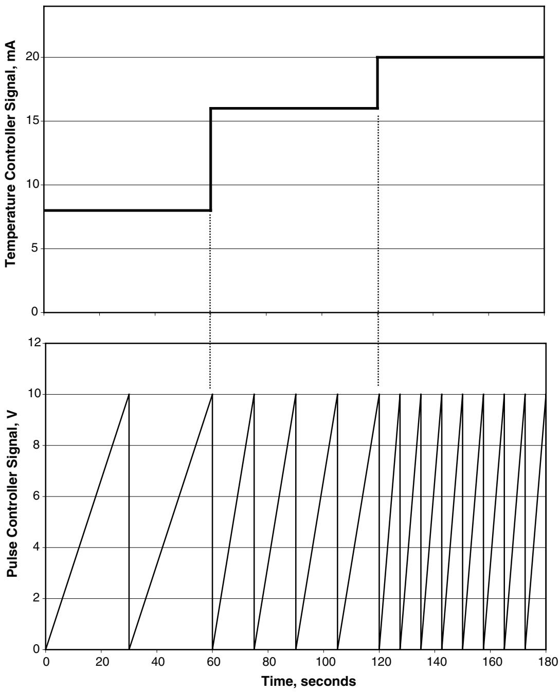
*Figure 4: Temperature controller signal conversion*
