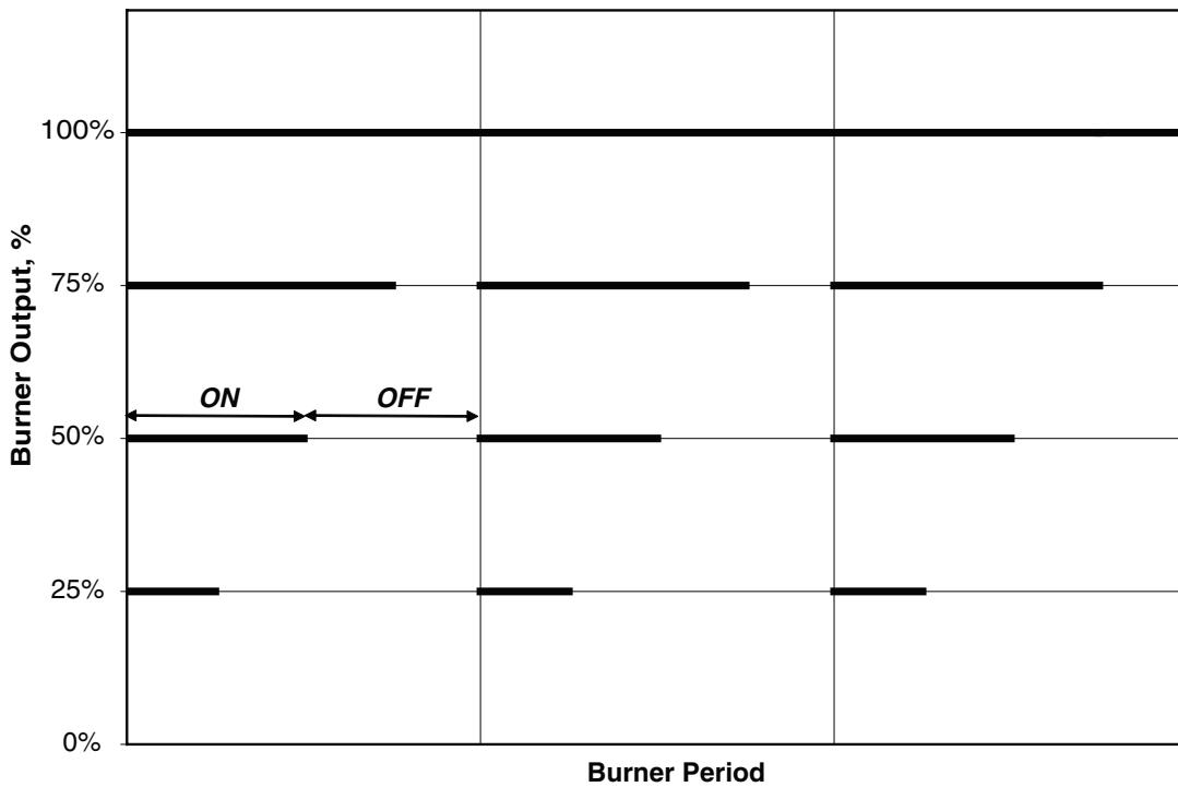
Figure 6: Burner period as a function of required output
