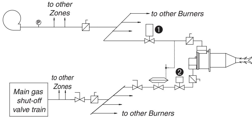
Figure 3: Typical on-off frequency-modulated combustion system
