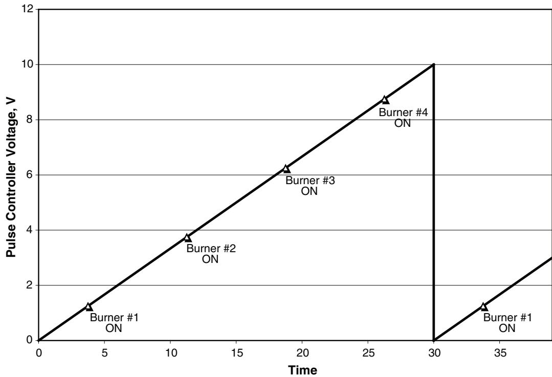
Figure 5: Example of trigger voltage assigned to a specific burner
