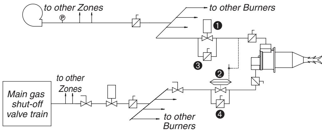
*Figure 2: Typical high-low frequency-modulated combustion system*
