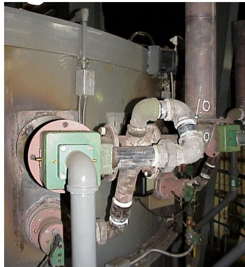
The South Coast Air Quality Management Department (AQMD) in California required that the total NOx production not be increased. The TFB075 burners alone were emitting around 75 ppm @ 3% O<sub>2</sub> (.091 lb/MMBtu) or .47 lb/hr NOx. The TFB burners with recuperators and FGR devices produced 45ppm @ 3% O<sub>2</sub> (.055 lb/MMBtu) or .40 lb/hr NOx.
