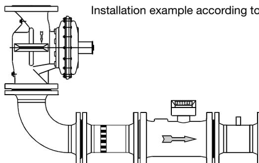
BLN 1 flow conditioner for installation in the inlet pipe and for use with high level perturbations
