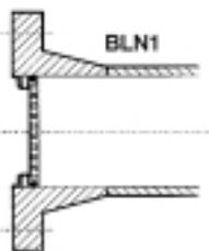
BLN 1 flow conditioners are inserted into the pipe, the best position being in the flange before the welding point (see sketch).
