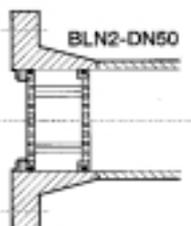
BLN 2, DN 50 flow conditioners are inserted into the pipe, the best position being in the flange before the welding point (see sketch).
