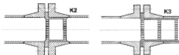
The K 2 and K 3 DN 50 – DN 400 flow conditioners are inserted into the pipe. Ensure that the welding joints (see sketch) near the flange/pipe transition do not extend too far into the pipe. Alternative flow conditioners are available to cater for the various thicknesses of the pipe walls.
