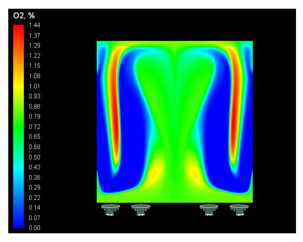
FIGURE 3: Oxygen Volume Concentration On Bath Surface.
