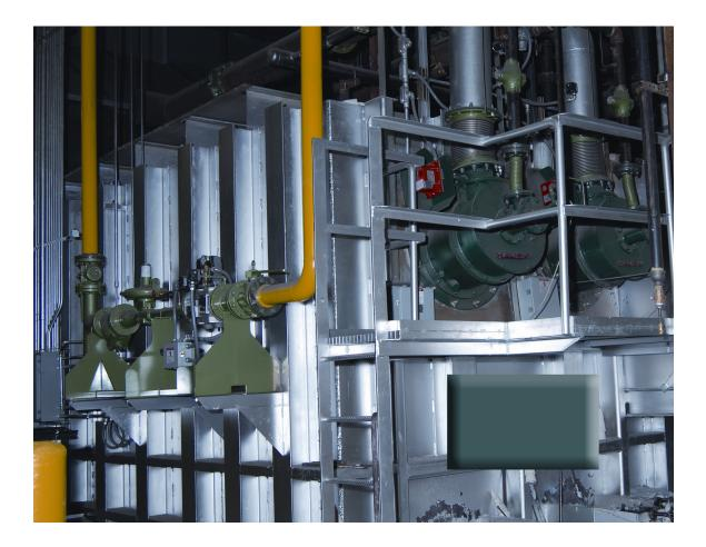
FIGURE 1: Side Well Melter, Main Chamber and Burners.
