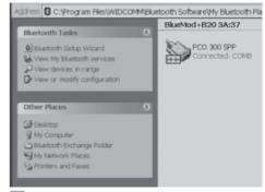
15 Confirm the link between the devices by clicking on "OK". ➤ This opens the "My Bluetooth Places" window and "PCO 300 SPP" is displayed.
