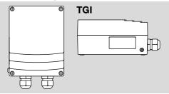
→ Position the ignition transformer right next to the burner (ignition cable length: max. 5 m, recommended < 1 m).
