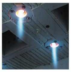
Overhead firing with BIC burners
