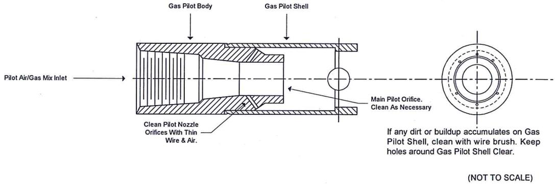
**Figure 3. Cleaning Pilot Nozzle and Piloting Holes**
